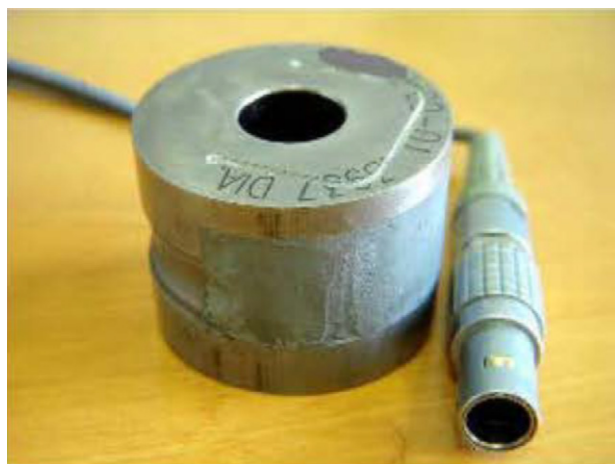
Fig. 1. An instrumented die.
